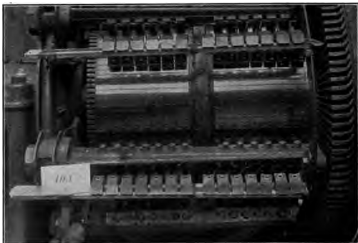
FIG. 92.—A later view of the commutator shown in Fig. 70 after operating with grooved mica. A perfect surface has been produced, free from roughness, ridges and blackened spots.
